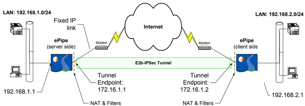
Figure 1 - Example network showing IP addressing.
